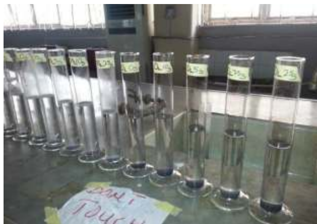
Figure 3b: Set of settling test cylinders
